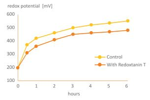
Increase in redox potential over time in a Tempranillo must. Control: Untreated must. With Redoxtanin T: dose of 8 g/100 kg.
